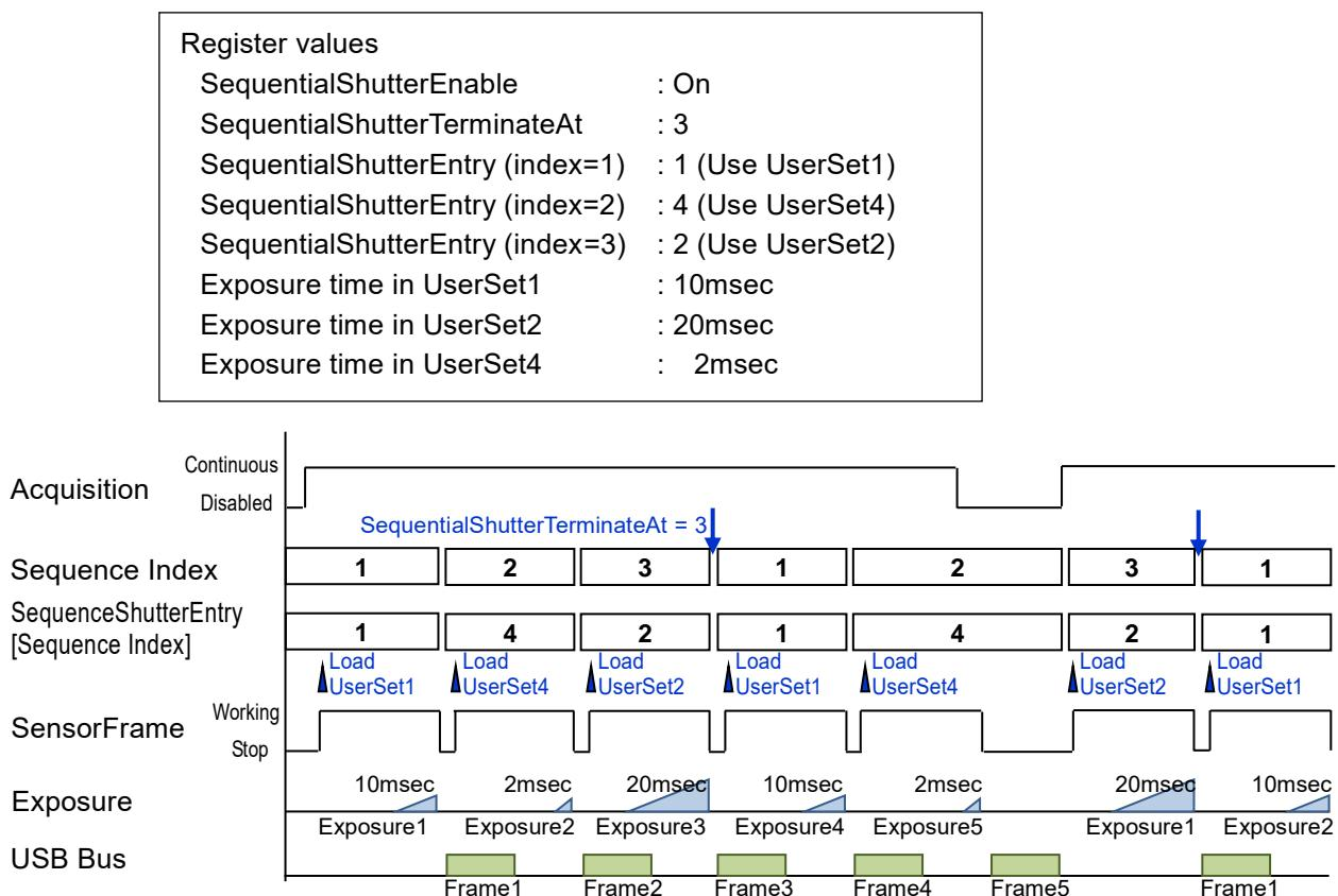
Note that sequence index starts from 1 and it will not be cleared to 1 even if image acquisition is stopped. Sequence index will be cleared to 1 by disabling SequentialShutterEnable and enabling it again during image acquisition is not active.
