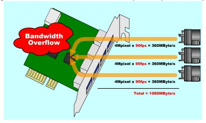
To solve this bandwidth overflow, the frame rate setting should be lowered to 30fps.
